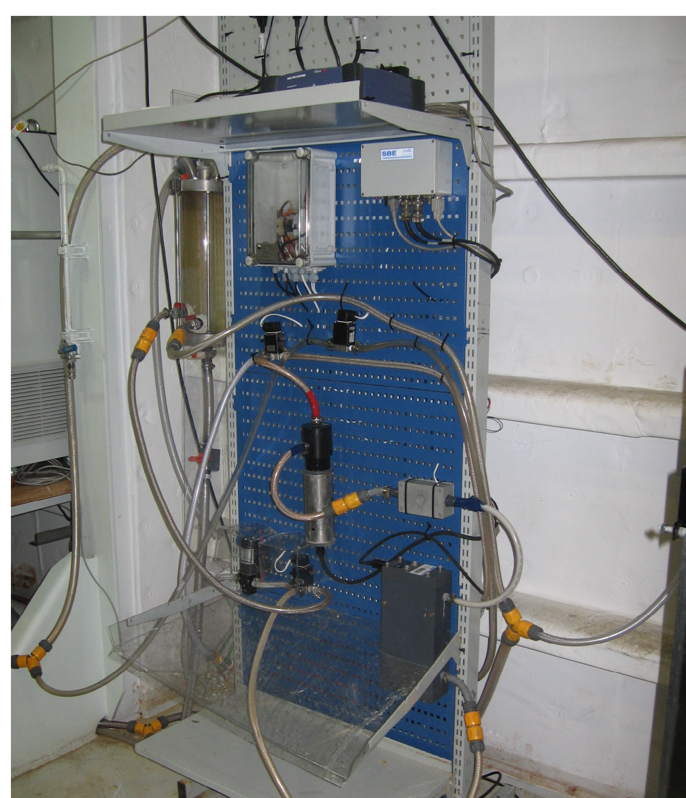
Fig. 3. The sensors on the ferry Finnmaid on the Helsinki-Lübeck route operated by FIMR. The system on TransPaper will be similar.
